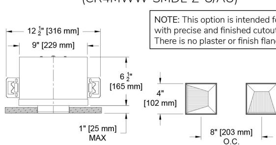
NOTE: This option is intended for use with precise and finished cutouts. There is no plaster or finish flange.
