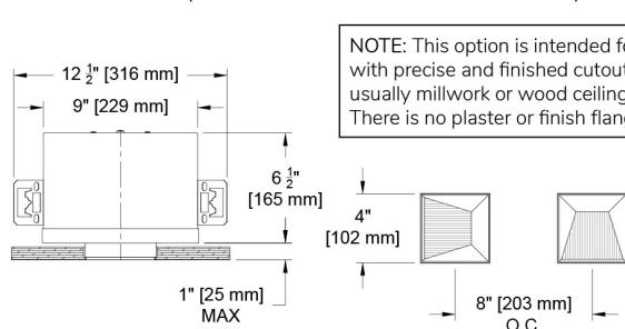
NOTE: This option is intended for use with precise and finished cutouts - usually millwork or wood ceilings. There is no plaster or finish flange.
